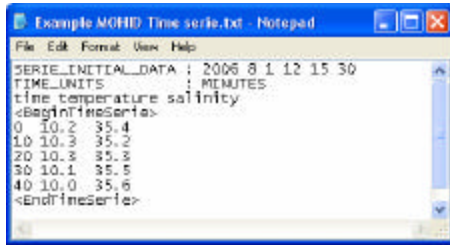
Figure 1. Example file of a MOHID Time series.
