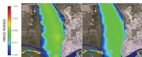
Figure 11. Velocity fields using bathymetry from Topo to Raster isotropic interpolation (left) and along-channel kriging (right).
