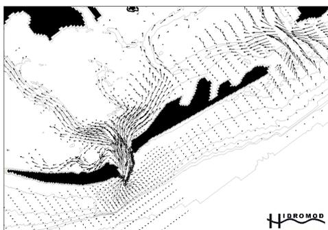
Figure 11: velocity patterns in a flood situation
