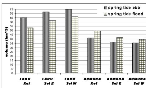
Figure 10 – Comparison of the tidal prisms for the Faro and Armona inlets considering the alternative solutions.
