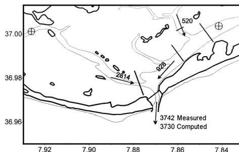
Figure 9: Comparison of the measured and computed Faro inlet water fluxes in spring tide ebb conditions (after IH, 2001)
