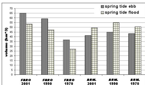
Figure 7 – Computed tidal prisms for the Faro and Armona inlets from 1970 till 2001
