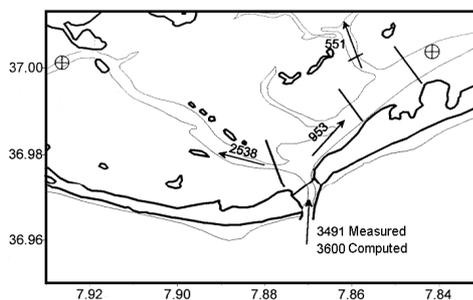
Figure 8: Comparison of the measured and computed Faro inlet water fluxes in spring tide flood conditions (after IH, 2001)
