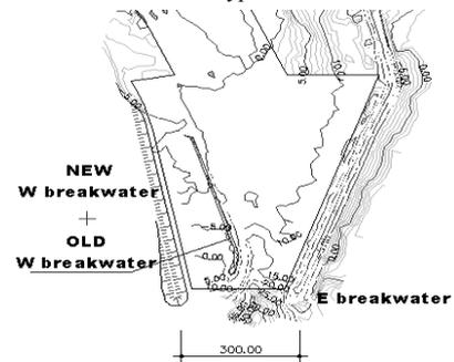
Figure 5: West breakwater type solutions
