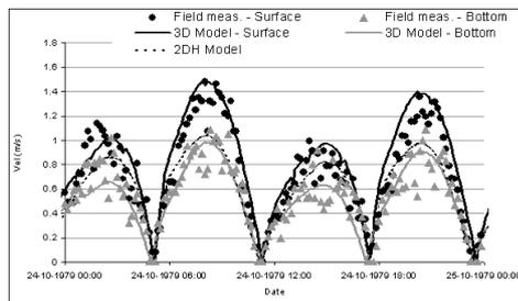
Figure 3: Comparison of measured and computed velocities at 2 depths in point 12.
