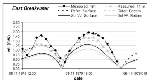
Figure 12: Comparison of measured and computed velocities at two depths, considering the reference situation and a West type solution.
