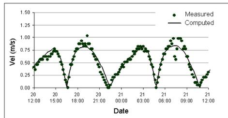
Figure 2: Comparison of measured and computed depth averaged velocities at point 3.
