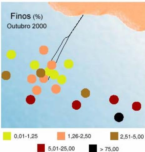
Figure 9: Distribution of fine material in October 2000, after 6 years of operation (Quintino *et al* 2000). Note that the scale is not exactly as in Figure 8.
