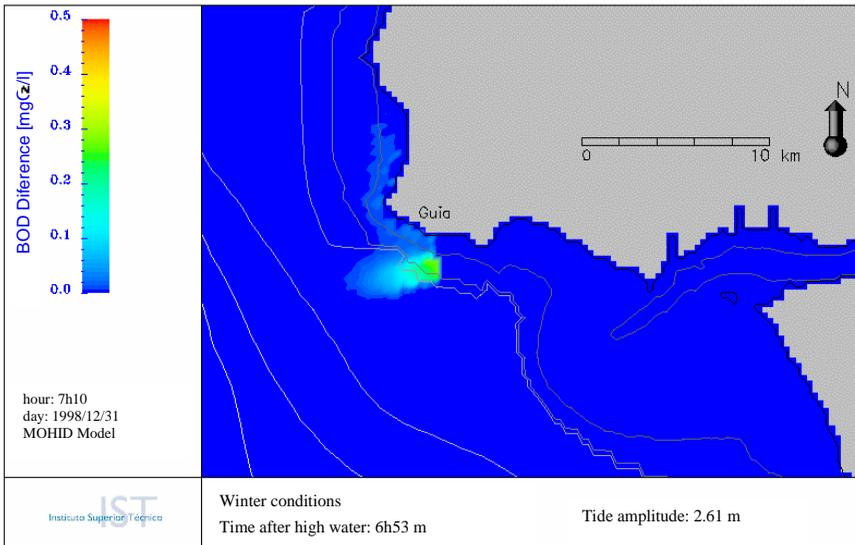
Figure 14: Differences between BOD concentrations in the water column, considering secondary and primary treatment.
