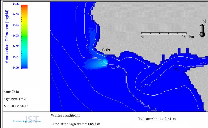
Figure 13: Differences between of ammonia concentrations in the water column, considering secondary and primary treatment.
