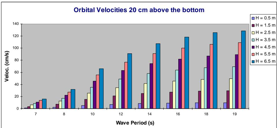
Figure 7: Orbital velocities generated by the waves 20 cm above the bottom, as a function of their period and height (Consulmar, 1996).
