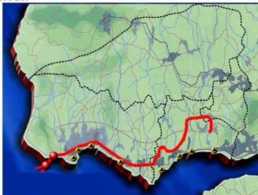
Figure 2: Schematic representation of “Costa do Estoril” sewage system. The gravity trunk sewer, ends at the treatment plant, which is followed by a 2750 m long submarine outfall.
