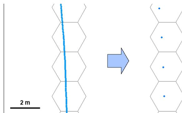
Figure 4. Aggregating bathymetry (initial data on the left and the result at the right side)
