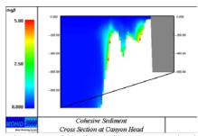
**Figure 6** – Cross section along the canyon axis showing the sediment concentration near the bottom.
