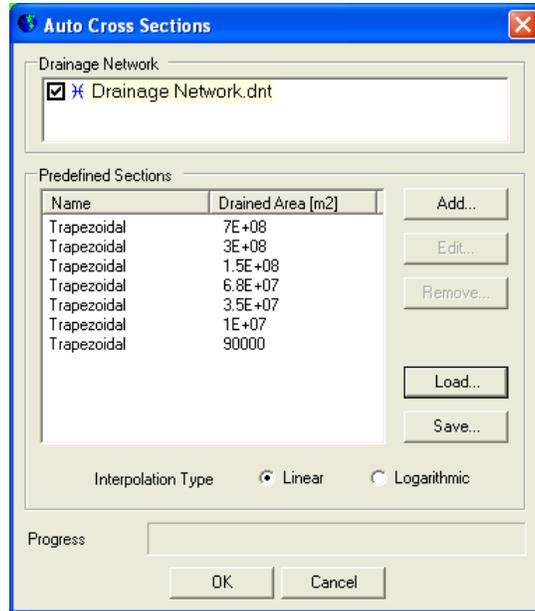
**Figure 3-26: Window to interpolate Cross Sections**
