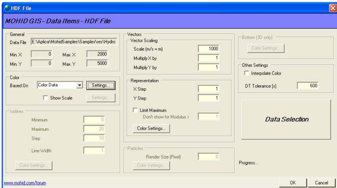
**Figure 3-14: Properties window of a HDF 5 Data Item after Data Selection**
