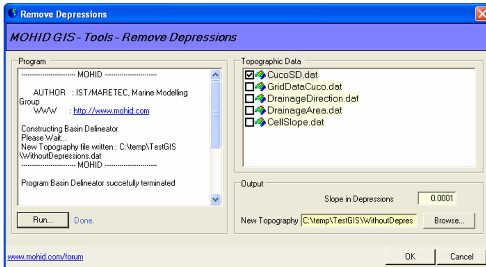
Figure 3-24: Window to Remove Depressions
