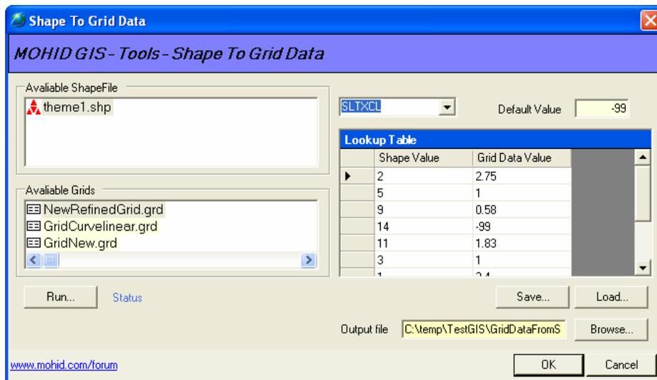
Figure 3-29: Converting Polygon Shape File into Grid Data
